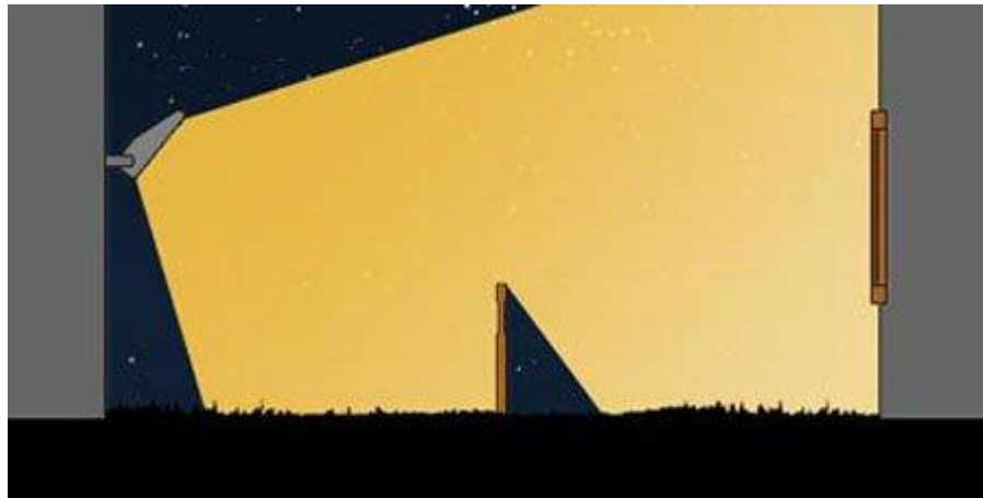
Figure 9.6: Light unit with environmental (cut-off) armature
